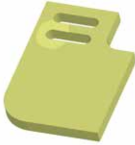
Potential Delamination with Standard Cutting Head: Scrap Part & Restart Production
